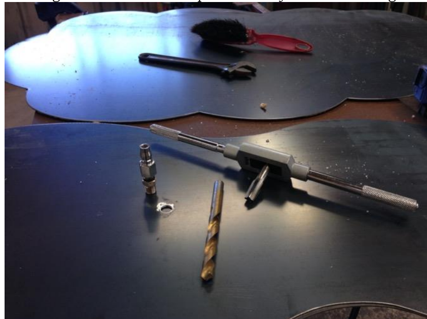
Figure 15: Valve preparation with tapped central thread
