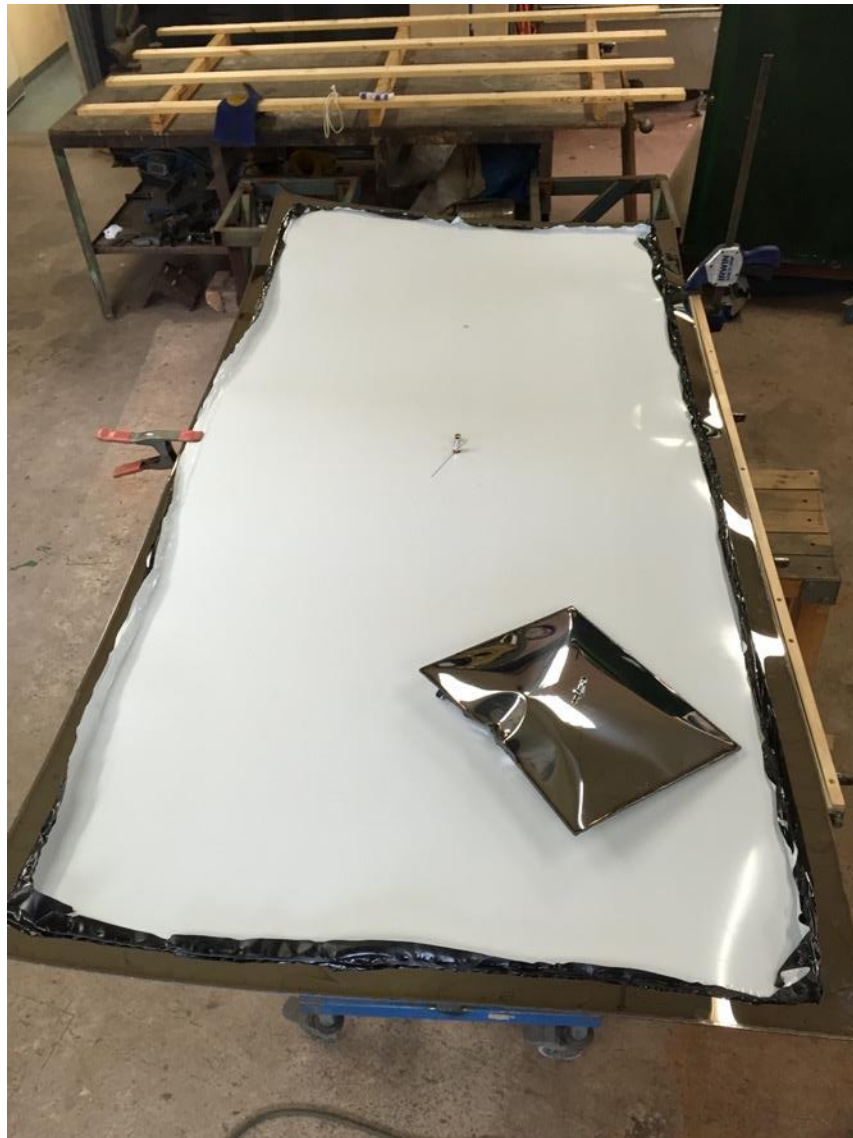
Figure 18: Work in progress. Image of test piece and completely welded final pieces ready for inflation at The Lockup.
